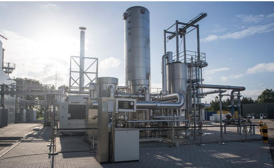
HZIBM amine scrubbing is a component of the power-to-gas plant in Werlte, Germany (Photo: Audi AG)
