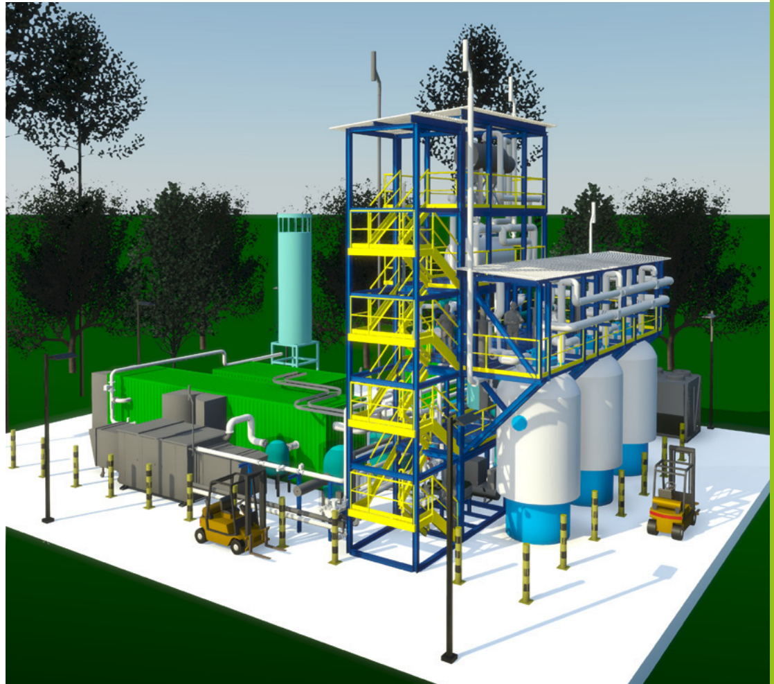
Pythia6000 – HZI catalytic methanation reactor series for 6000 Nm 3 /h feedgas
